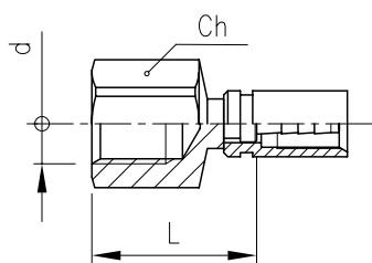
**Manometeradapter****Female fixed thread fitting****Schlauchart / Hose type****6400**
